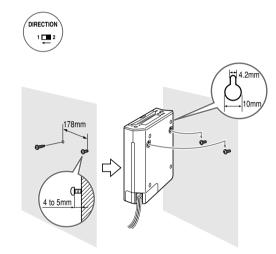
Mount two commercial screws onto the wall with each screw located in the same height.
